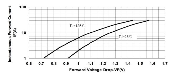
Fig.3-Typical Forward Voltage Drop Characteristics
